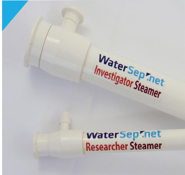
Designed for perfusion and aseptic applications, WaterSep's **Steamer Line** autoclavable hollow fiber cartridges are gamma irradiated and ready to use. They do not contain humectant and are pre-wetted with deionized water so minimal flushing is needed before use. The cartridges can be cleaned, stored and autoclaved up to five (5) times.
