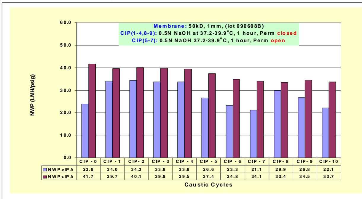
In Figure 1, the NWP profile is presented for the “test” element measured before and after each caustic cycle. NWP results measured after IPA exposure showed a stable profile that leveled off to a maximum NWP reduction of 19%. This change is still well within the permeability specification. NWP results measured before IPA showed a smaller decrease (6%) from initial to final cycle but with a higher expected standard deviation. Thus, more weight is always given to the NWP after IPA.
