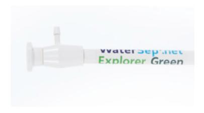
The Explorer<sup>™</sup>41 Green hollow fiber membrane cartridges are designed for laboratory scale biopharmaceutical applications for volumes that range from 300 mL to 3000 mL, with a final retentive volume of less than 35 mL. The Explorer<sup>™</sup>41 Green cartridges have a membrane surface area of 579 cm², providing an average permeate flow rate of 1.7-3.5 L/hr for ultrafiltration applications and 1.2-2.3 L/hr for microfiltration applications.
