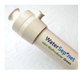
The mini-BioProducer Green hollow fiber cartridges are designed for pilot and small production scale and are the perfect tools for process development. With a surface area of 0.63 m², the mini-BioProducer12 Green HF cartridge can accommodate batch volumes between 5L and 50L with a typical permeate flow rate of 18.9-37.8 L/ hr for ultrafiltration applications and 12.6-25.2 L/hr for microfiltration applications.
