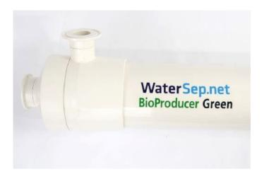
The BioProducer Green production scale hollow fiber cartridges are designed for biopharmaceutical concentration/diafiltration and clarification unit operations. With a surface area of 5.0 m², the BioProducer41 Green HF cartridge can accommodate batch volumes between 100L and 500L with a typical permeate flow rate of 150 to 300 L/hr for ultrafiltration applications and 100 to 200 L/hr for microfiltration applications.
