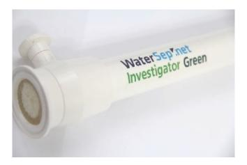
The Investigator Green crossflow hollow fiber membrane cartridges are designed for pilot scale and small scale production and is the perfect tool for process development. With a surface area of 0.27 m², the Investigator24 Green can accommodate batch volumes that range from 2L to 12L with a typical permeate flow rate of 8.1 to 16.2 L/hr for ultrafiltration applications and 5.4 to 10.8 L/hr for microfiltration applications.
