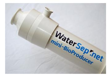
The mini-BioProducer41 ReUse series of cross flow hollow fiber membrane cartridges are designed for pilot scale and medium scale production and is the perfect tool for process development. With a surface area of 2.5  $\mbox{m}^2$ , the mini-BioProducer24 ReUse can accommodate batch volumes that range from 40 L to 250 L with a typical process flow of 125 L/hr.
