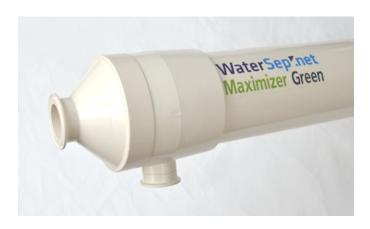
The Maximizer Green production scale hollow fiber cartridges are designed for biopharmaceutical concentration/diafiltration and clarification unit operations. With a surface area of 5.1 m², the Maximizer24 Green HF cartridge can accommodate batch volumes between 100L and 500L in a single cartridge system, and several thousand liters with a multi cartridge set up. It has a typical process flow rate of 153-306 L/hr for ultrafiltration applications and 102-204L/hr for microfiltration applications.
